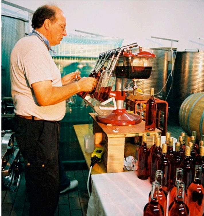
A small bottling room is located along side of the wine cellar. We have always filled the bottles manually, but we cork and label them with the help of machines.
