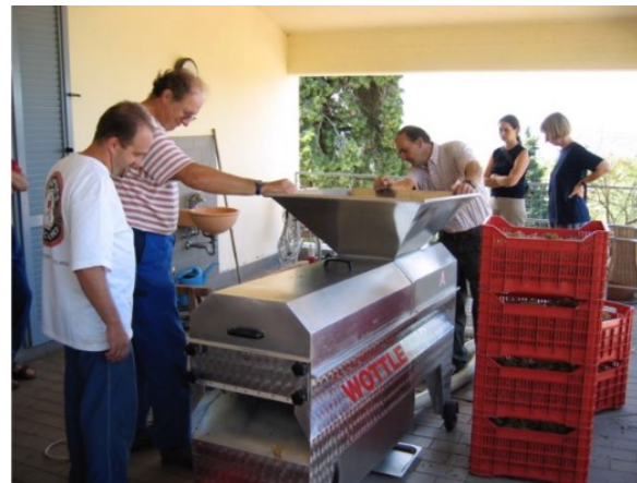
Grapes are separated from their stems, then sent down to ferment in steel tanks
